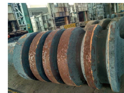
The grooved cast roll in as-cast condition
